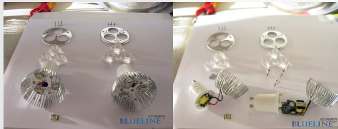
Removed PCB and power supply
